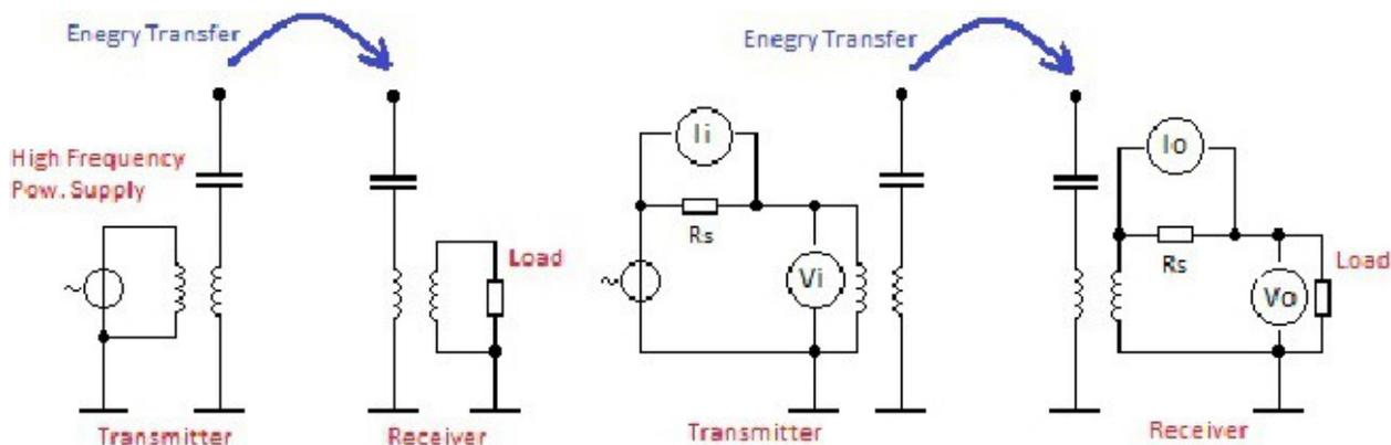
The circuit diagram of the Tesla coils including a measurement
