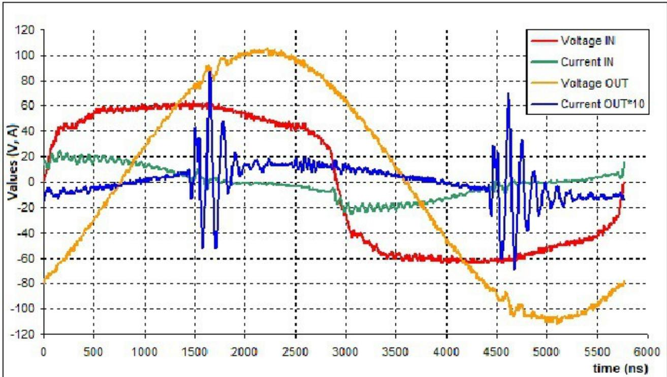
The measured input and output values
