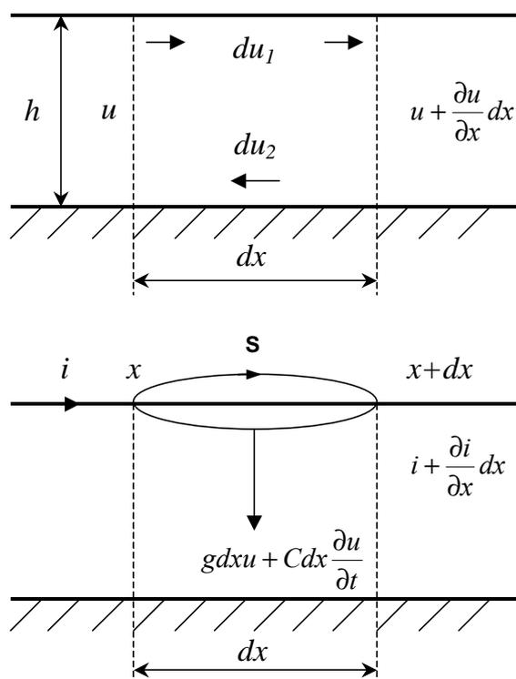
Fig. 2. Currents and voltage drops in single-wire line
