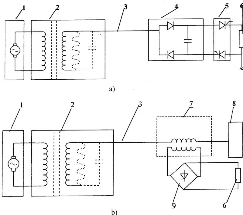
Fig. 1a. Low voltage single-wire line 10–1,000 V
