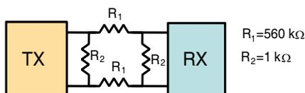
Figure 1: Calibration network.
